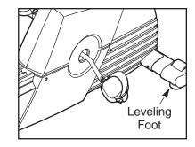
ly during use, turn one or both of the leveling feet under the front stabilizer until the rocking motion is eliminated.
